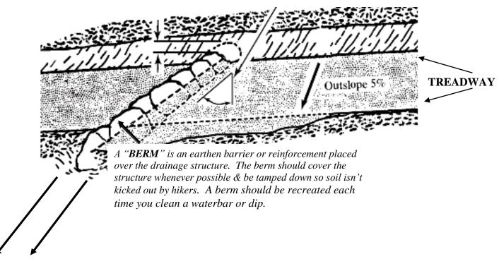
**OUTFLOW**=extension of drainage off the treadway
